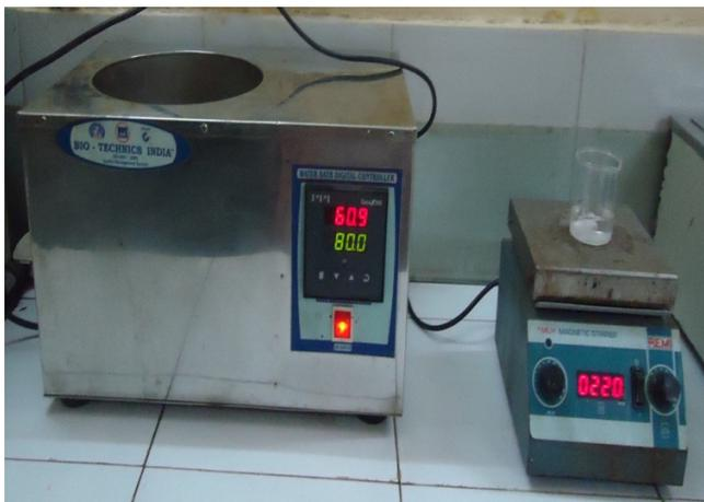
Among novel wet-chemical processes, the Chemical Bath Deposition method is used to synthesize nanoparticles more easily than the other method.
