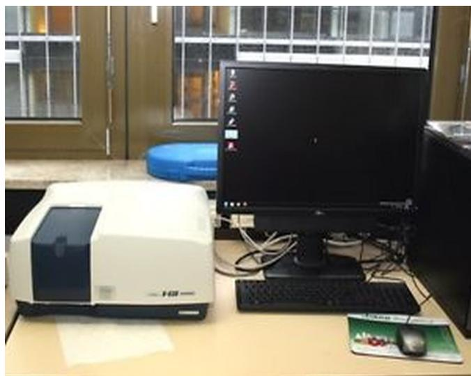
**Jasco Make Model:V-630-** for powder and thin film
